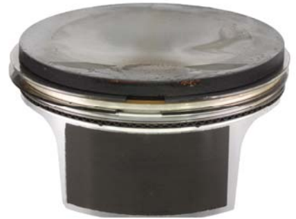
Pistons look great with minimal depositing on the crown.
