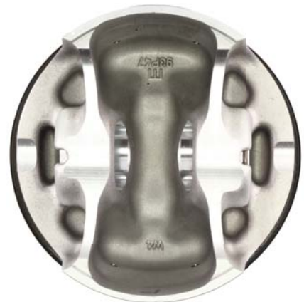
Piston undercrowns look almost new with no deposits or staining.
